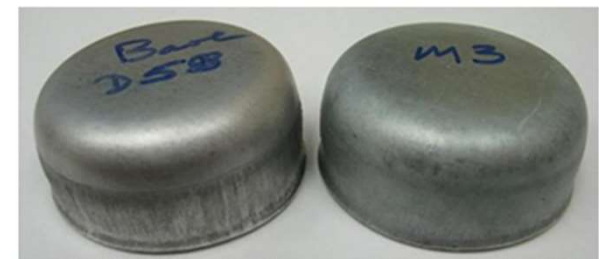
Liquid lubricant vs. Dry lubricant comparison on steel sheet
